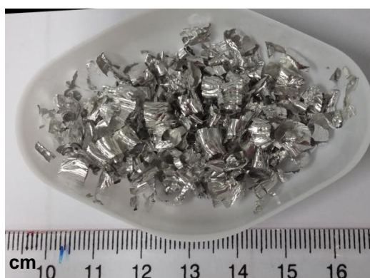
Fig. 1. Visual appearance of 0.5 g of testing materials with the surface area of 400 cm 2 /g.
