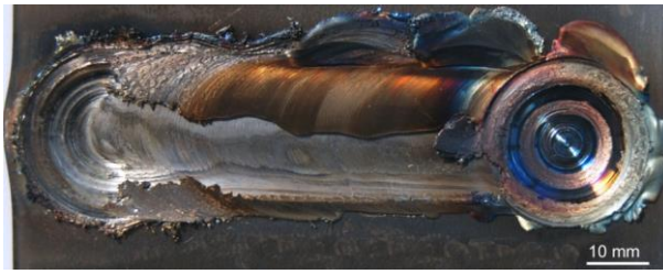
Fig. 2. Inadequate weld appearance obtained when placing 304SS as upper workpiece.
