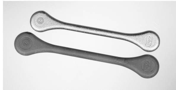
Fig. 2. MIM tensile test specimens referring to ISO 2740 (sintered and green part), total length of the green part was 90 mm.
