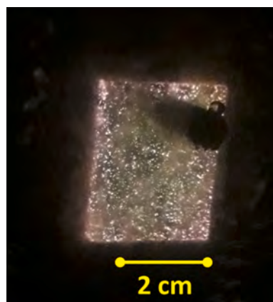
Fig. 4. Intense micro-discharges on surface of the metal alloy substrate during PEO processing in stage III.
