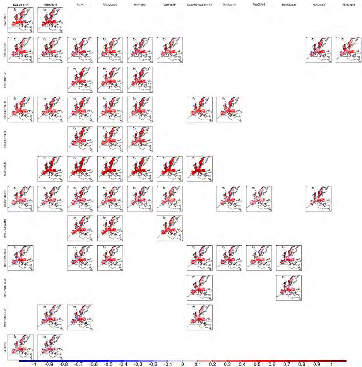
Fig. 7. Added value for 99-100 percentile fraction of the EUR-11 ensemble members compared to the ECO at a resolution of 0.11°.
