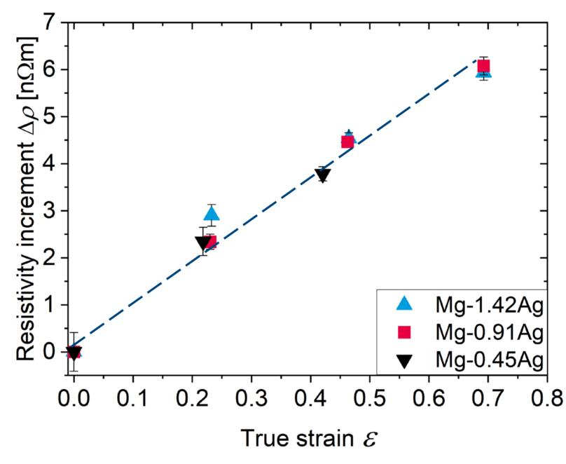
With increasing plastic strain, the concentration of crystal defects such as dislocations increases.
