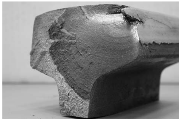
Figure 27: Fracture of a rail with origin from a head check. The rail was broken up in the laboratory.
