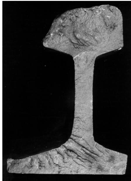
Figure 44: Fracture of rail caused by a corner crack at the foot.
