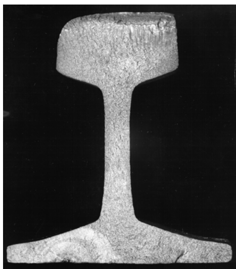
Figure 40: Rail foot crack starting from a corrosion pit at the foot underside.
