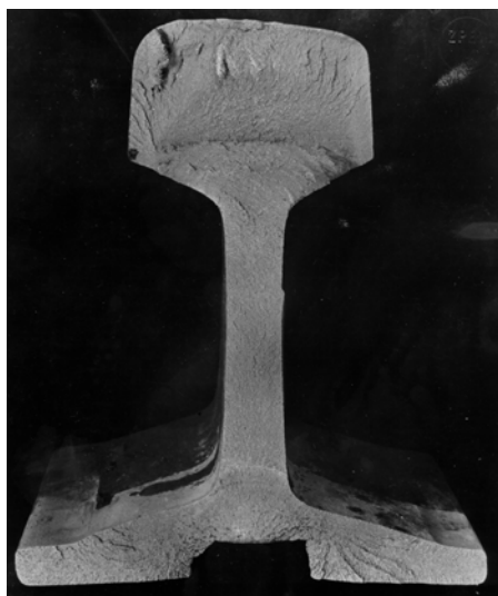
Figure 43: Fracture of rail caused by a crack which initiated at a cutout at the foot underside.
