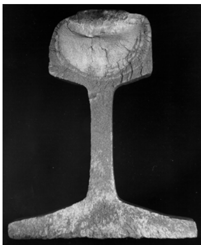
Figure 32: “Kidney-shaped” crack in a rail head.
