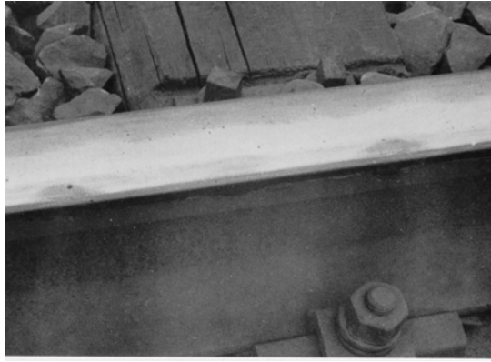
Figure 33: Gauge corner shelling at an early stage.
